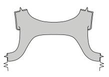
7. Open out facing at shoulders. Pin front and back together, pin facing edges together. Stitch in one continuous seam.
